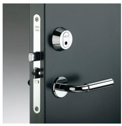
ABLOY® EL544 is a fast motor lock with dead bolt and handle-operated mechanical anti-friction latch bolt for wooden and steel doors.
